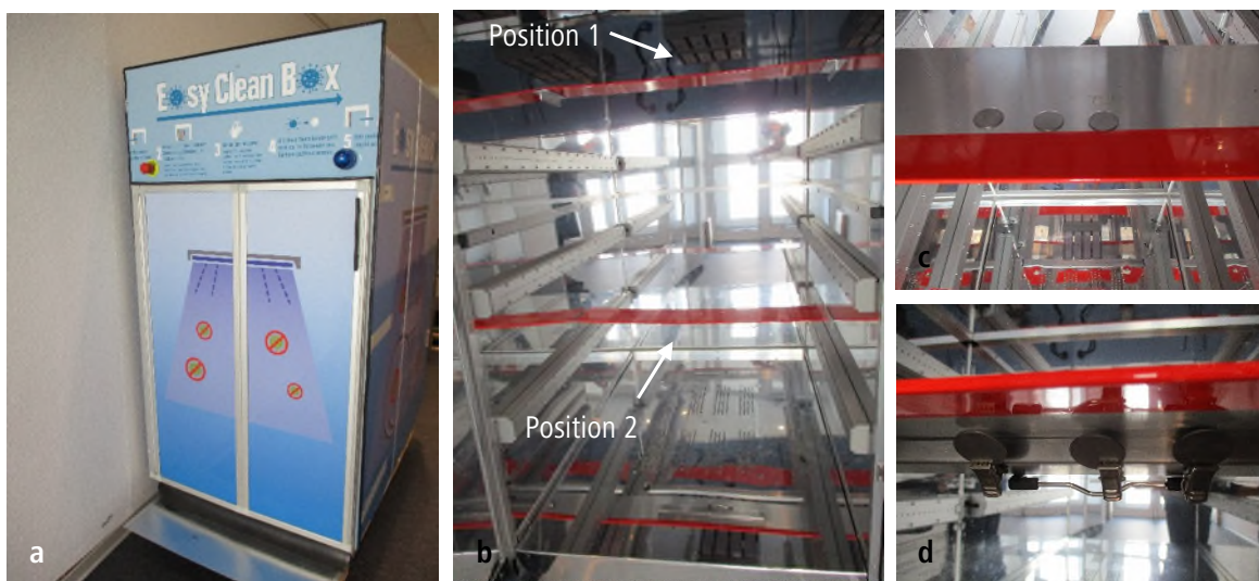
Figure1: Easy Clean Box EKW-UVC (a), inside (b) with the two tested positions. Position 1 on the upper plate (c) and position 2 at the lower plate (d)
